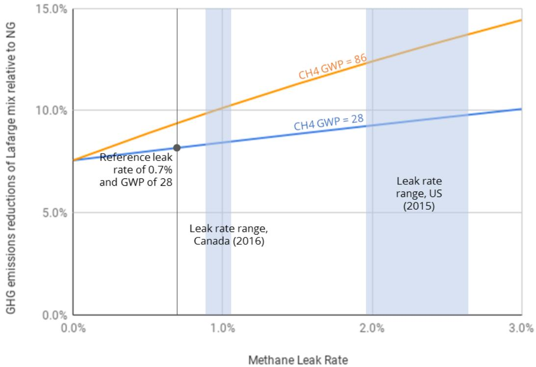
Figure 10. Trend in life cycle GHG reduction per tonne of clinker for the Lafarge fuel mix relative to natural gas with a varying methane leak rate for 20 and 100-year methane GWPs.
