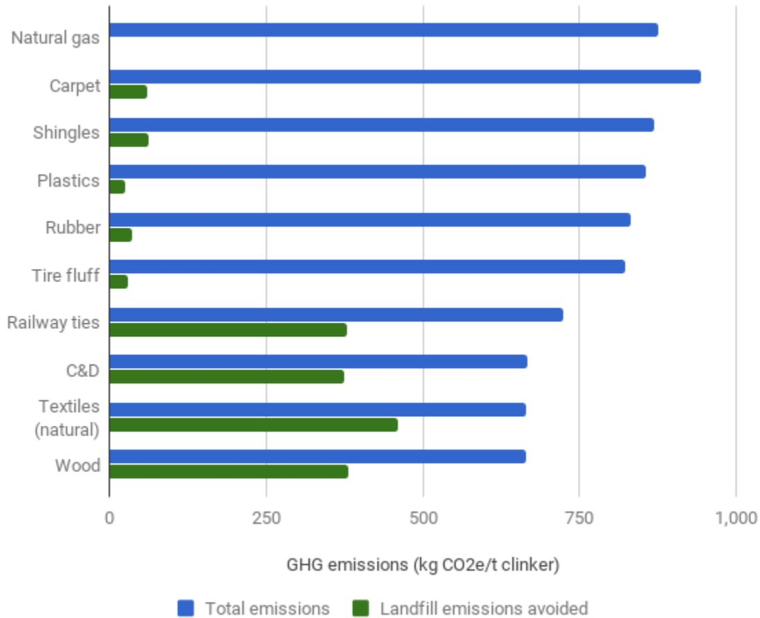
Figure 5. Total GHG emissions per tonne of clinker and avoided landfill emissions for natural gas and alternative fuels assuming a 100% fuel substitution rate
