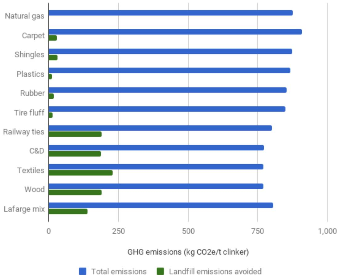
Figure 8. Total GHG emissions per tonne of clinker and avoided landfill emissions for natural gas and alternative fuels assuming a 50% fuel substitution rate.
