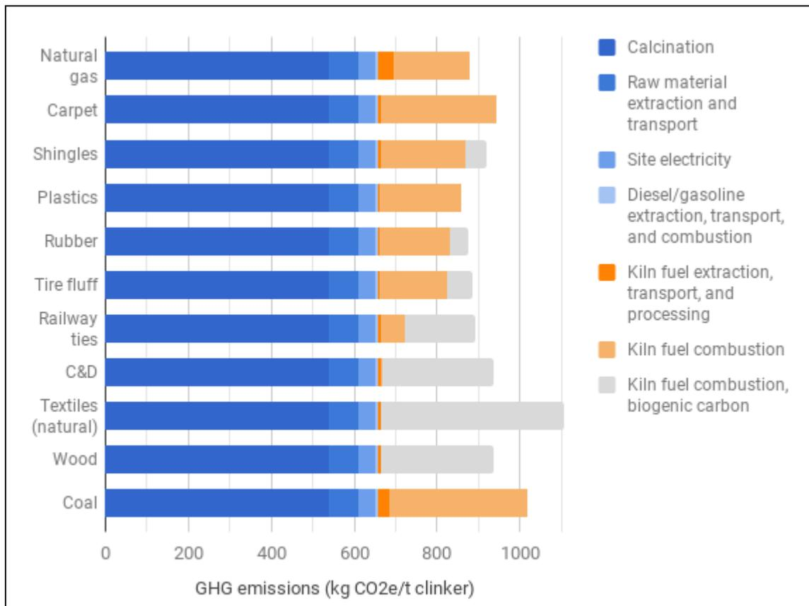
Figure 3. Comparison of GHG emissions per tonne of clinker for natural gas, coal, and alternative fuels assuming a 100% fuel substitution rate
