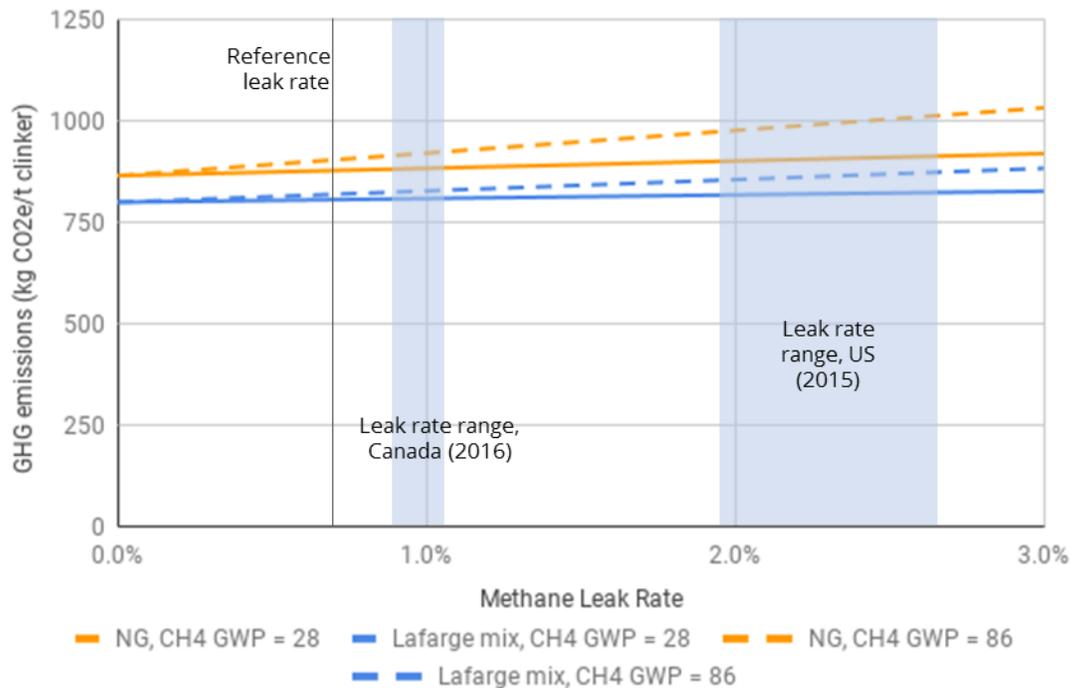
Figure 9. Variation in total GHG emissions per tonne of clinker for natural gas and the Lafarge fuel mix with methane leak rate for 20 and 100-year methane GWPs.
