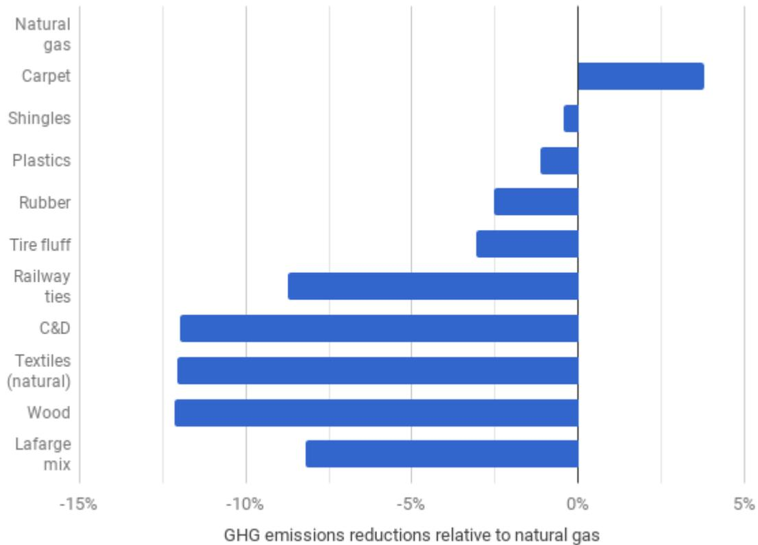
Figure 7. Comparison of GHG emissions per tonne of clinker of coal and alternative fuels against natural gas assuming a 50% fuel substitution rate
