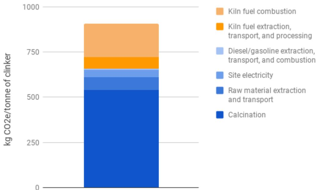
Figure 2. Breakdown of life cycle GHG emissions per tonne of clinker for baseline scenario
