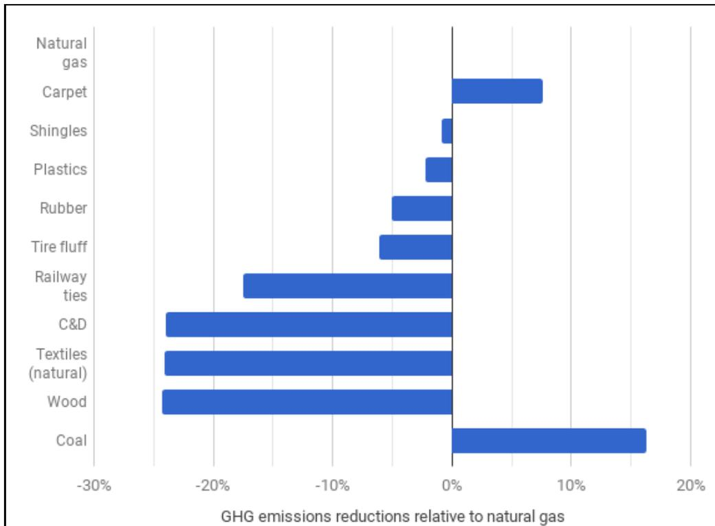
Figure 4. Comparison of GHG emissions per tonne of clinker of coal and alternative fuels against natural gas assuming a 100% fuel substitution rate
