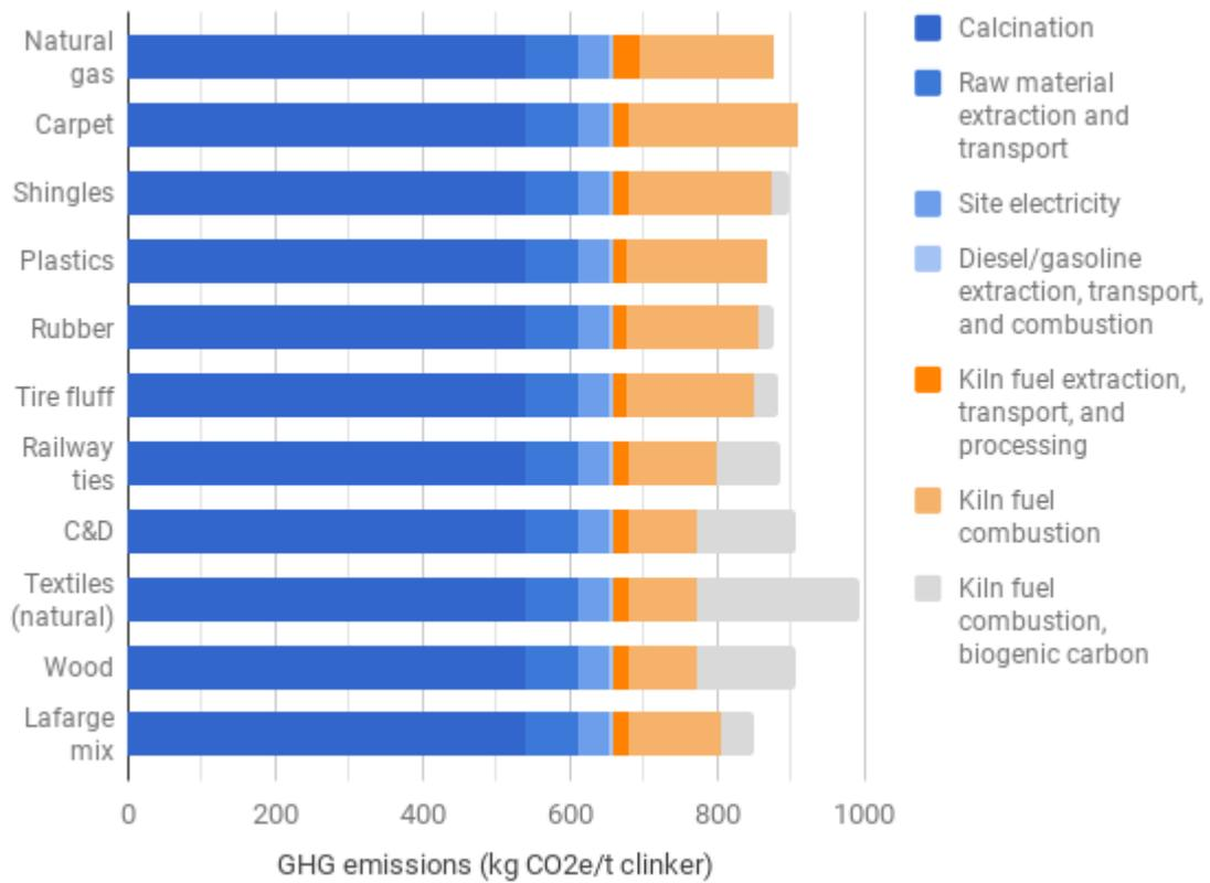
Figure 6. Comparison of GHG emissions per tonne of clinker for natural gas and alternative fuels assuming a 50% fuel substitution rate
